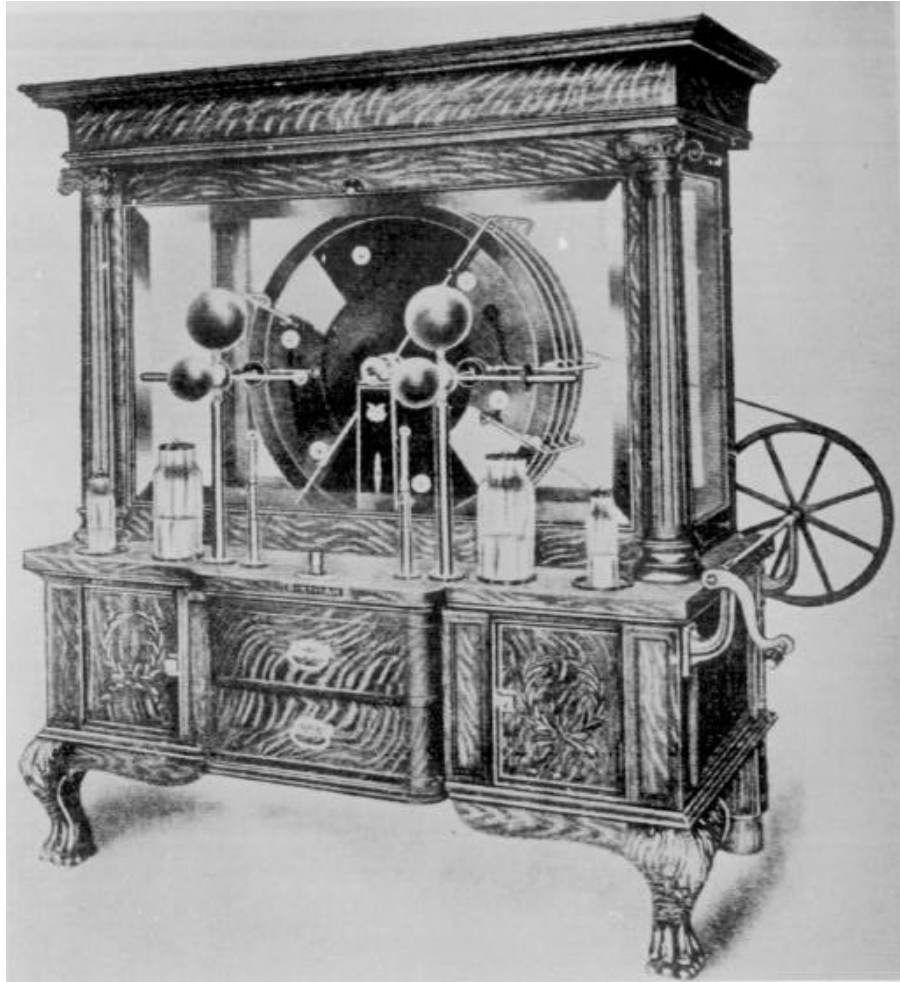
Fig. 1.1 Model of hand-operated Wimshurst friction generator
